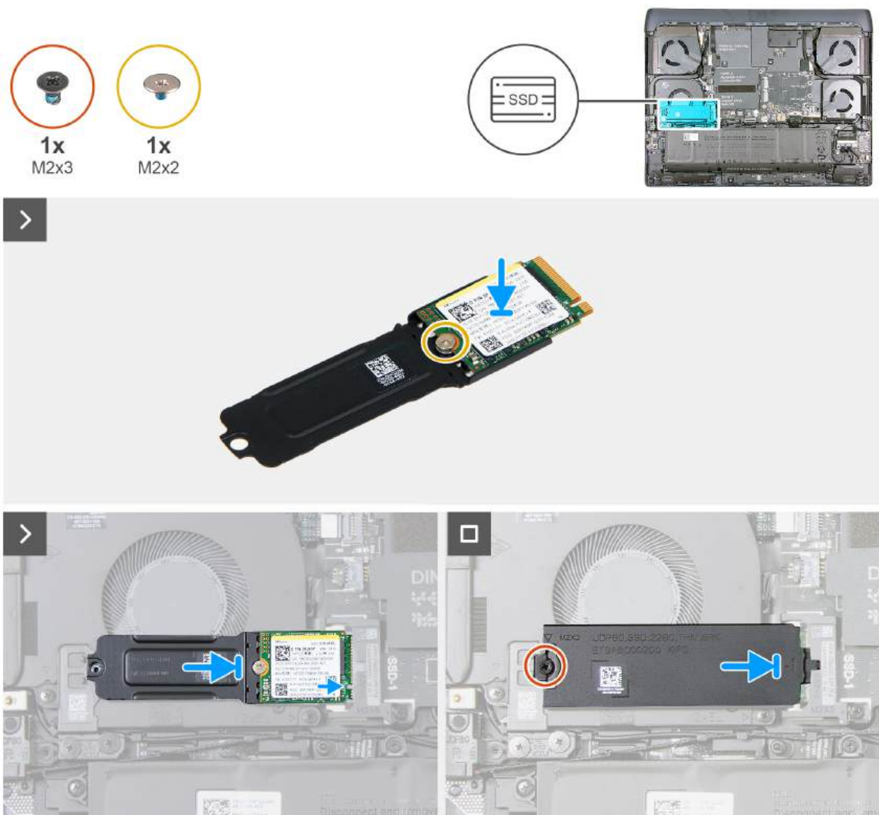
Figure 24. Installing the M.2 2230 SSD in slot 1
